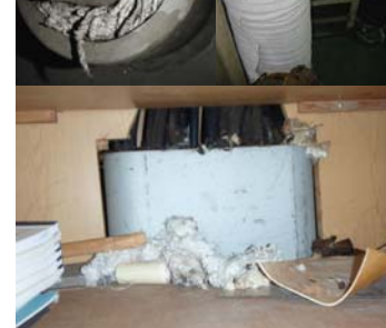
Above and right: asbestos can be found in all sorts of locations onboard, including insulation, bulkheads, flooring and packings. Pictures: Oesterbaai
